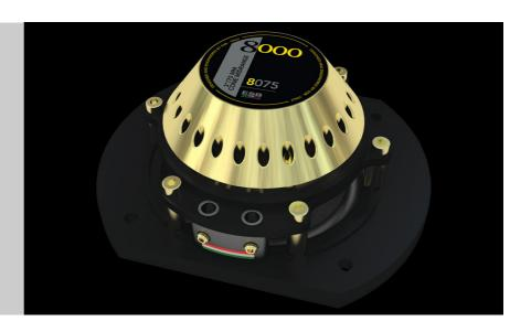
Neodymium magnet motor is optimized with FEA simulation to ensure perfectly symmetrical magnetic flux in both directions of the cone's run. Motor metal parts are CNC machined from solid and refined material for maximum magnetic flux linearity and minimum magnetic loss. This reduces distortion at high power levels.
