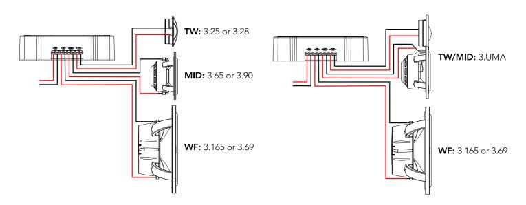
It is absolutely vital that your component system must be connected as shown in this manual. If not connecting the system as shown may cause damage to speakers NOT covered by warranty. Do not change different crossover networks or speakers, this crossover is specially designed for 3000 series speaker system. Do not use crossover networks intended for several ESB series models unless expressly indicated.
